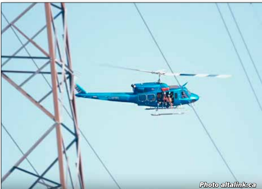
A crew checks the status of a line from the air.
